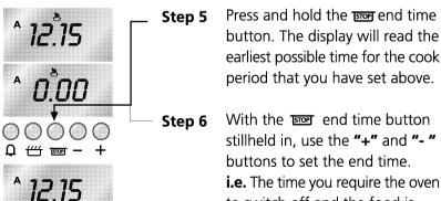
With the **low** end time button stillheld in, use the "+" and "-" buttons to set the end time. **i.e.** The time you require the oven
