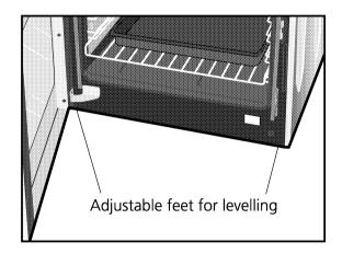
Lift the front feet clear off the floor by lifting at the ends of the hotplate fascia.
